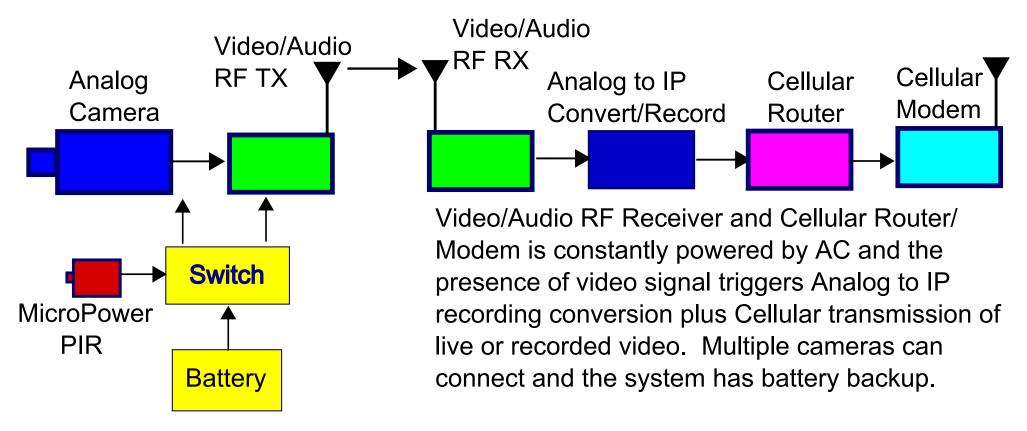
A MicroPower PIR turns on power for an Analog camera and Analog RF Transmitter for a timed event period. The advantage is that an Analog Camera is "Instant-On" from a powered off state, versus an IP camera with a "boot time", allowing for extended battery operation or indefinite, unattended operation with solar charging. An additional transmitter can be added to poll for supervised operation.
